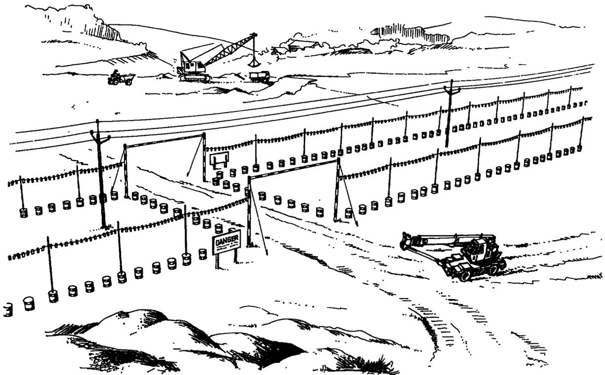
**Figure 2:** Sites where plant will pass under the line. Example of rigid goal posts and barriers. Similar precautions apply to lines supported on steel towers.
